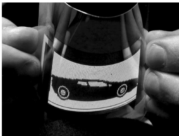
Fig. 5. 128 \times 64 passive matrix (60 dpi) monochrome green PHOLED display fabricated on barrier coated 0.175-mm heat stabilized PET (courtesy of Universal Display Corp.).
