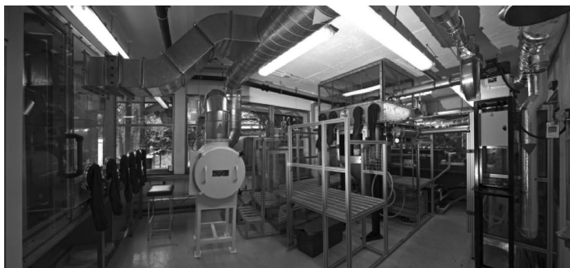
Figure 4. A flame aerosol reactor pilot plant at the Johnson Matthey Research Center, UK. This plant offers synthesis of various nanoparticle compositions by flame spray pyrolysis within the NanoCentral alliance ( www.nanocentral.eu ).
