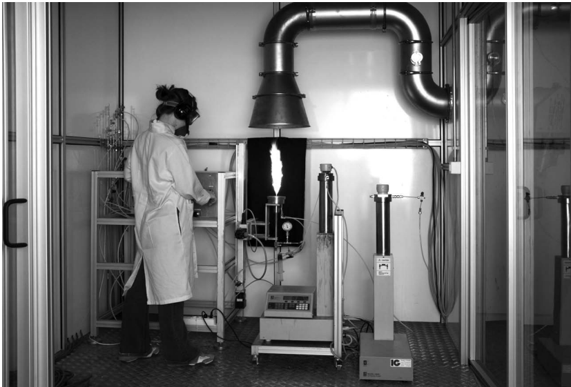
Figure 5. A flame spray pyrolysis aerosol reactor at the Swiss Federal Institute of Technology (ETH Zurich) for continuous synthesis of mixed noble metal and ceramic nanopowders up to 1 kg/h.
