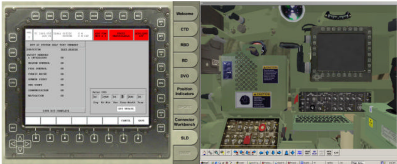
Figure 6: The M2A3/M3A3 VR DT uses a combination 3D and 2D displays where the 2D display is driven directly by the tactical software.
