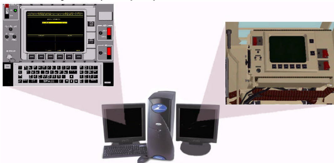
Figure 2: The VR DTs use two screens: one is a high-resolution 2D touch-screen for displays and interactions and a second for the 3D view of the vehicle
