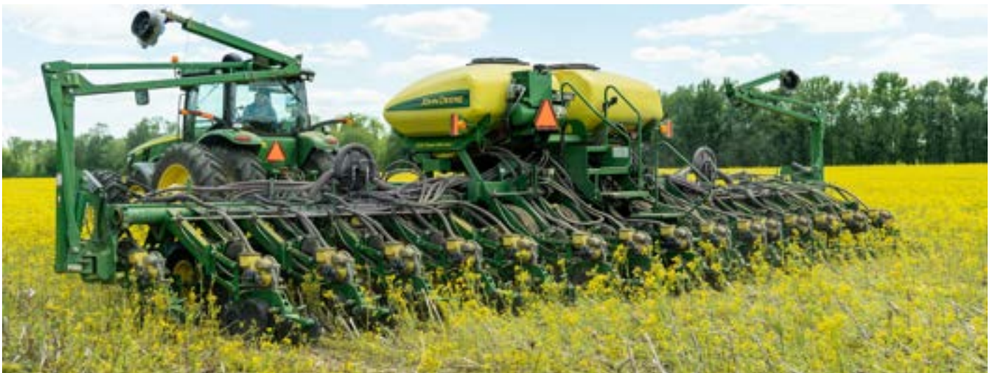
Planting soybeans into corn residue and wild mustard using a no-till planter on a farm in Vincennes, Indiana, on May 13, 2021. (Indiana Natural Resources Conservation Service photo by Brandon O'Connor)
