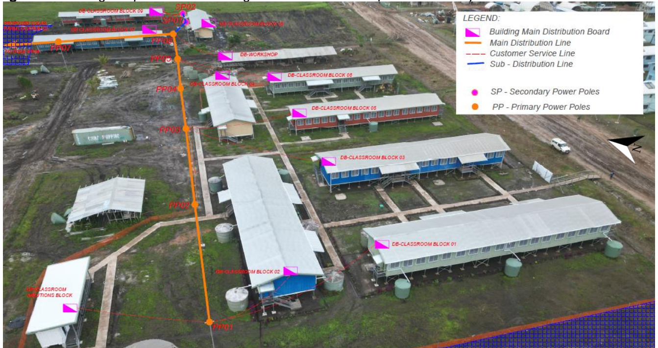
Figure 17. Existing and planned distribution grid towards north side of Balimo Academy
