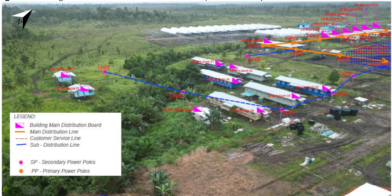
Figure 18. Existing distribution reticulation towards west side of Balimo Academy
