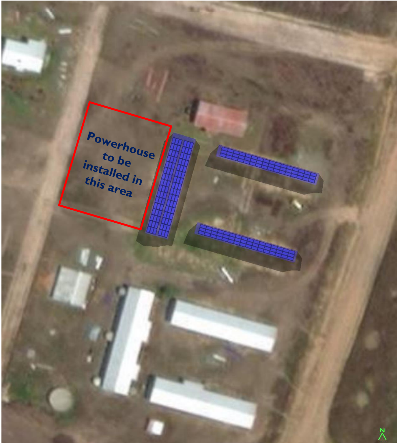
Figure 21. Indicative 96 kWp solar PV layout design on the classroom blocks 04, 05 and 06 and location where the powerhouse is to be installed
