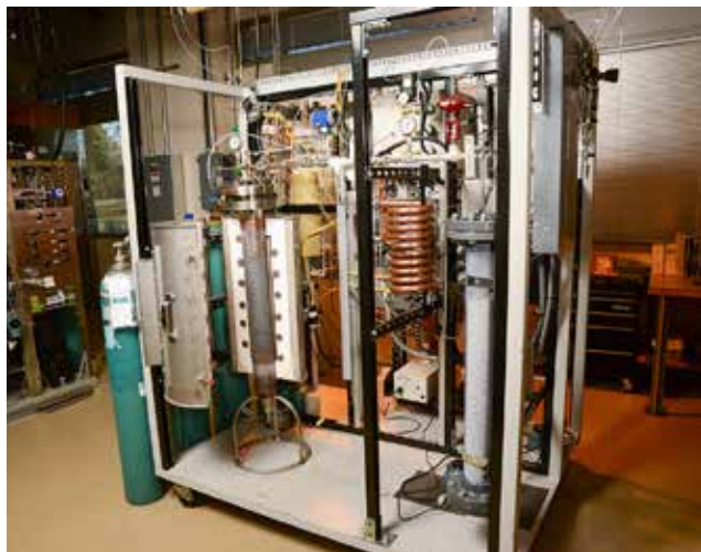
High-pressure, high-temperature fluidized-bed reactor
