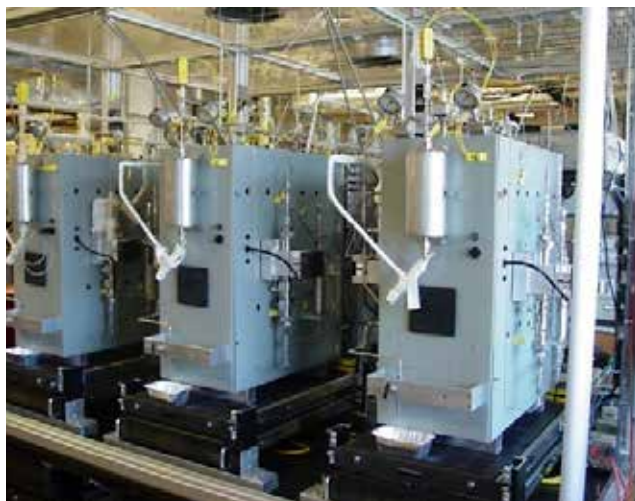
Lab-scale automated micro-reactor systems
