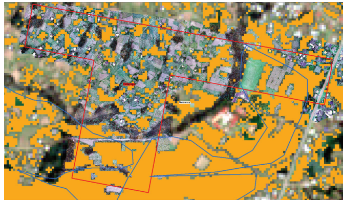
This image shows maize classification on the satellite Sentinel 2 imagery at a 10-meter resolution. The part outlined in red shows drone imagery overlaid on the satellite imagery at a resolution of 3–5 centimeters. Using this information, we can calculate—at a national scale—how much land is growing maize.
