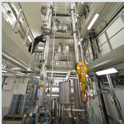
Emissions Control Tiller, 2018+ Effective emissions mitigation strategy for water lean solvent (WLS) at engineering-scale 1 t/day
