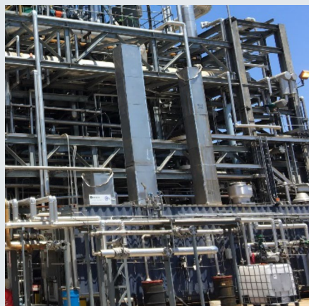
Pilot Testing at SSTU (Slipstream Solvent Test Unit) National Carbon Capture Center, 2018 Degradation, emissions, and corrosion characterizations under real flue gas 580 hours testing using coal power plant-derived flue gas 1 t/day
