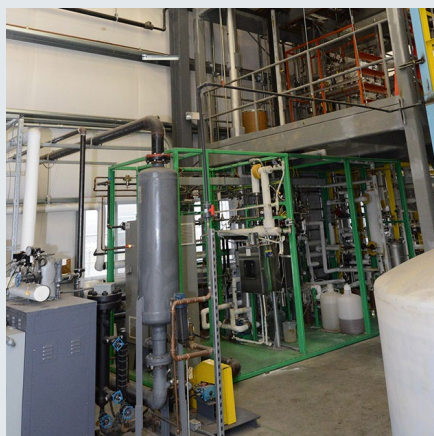
Large Bench-Scale System RTI Facility, 2014–2016 Testing of key process features ( \leq 2.0 GJ/t CO 2 ) at bench scale 1,000s of hours testing 0.1 t/day
