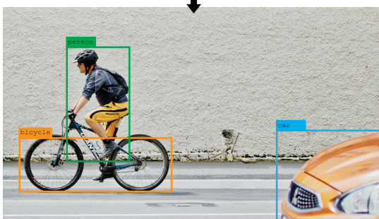
Figure 3: Each grouped region is classified as a single object. The narrowed focus of the analysis allows more efficient use of processing power, allowing the YOLO method to work in real-time.
