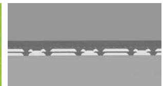
Two-layer Cu redistribution with two planar ILD layers
