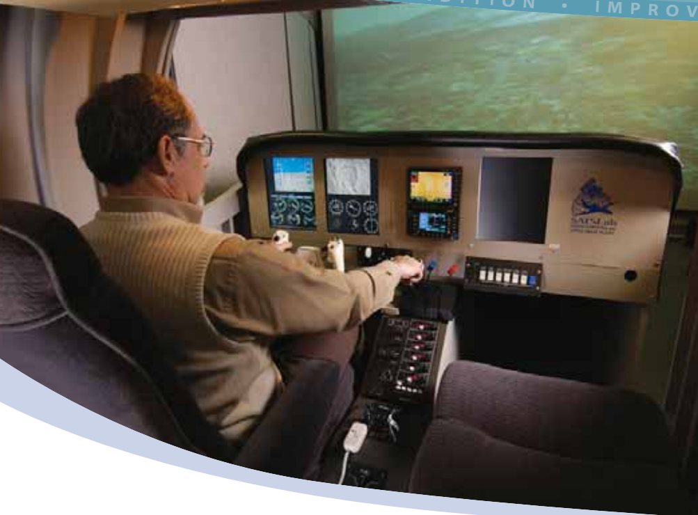
< Computer scientist James Henion demonstrates a flight simulator used to develop and test RTI's synthetic vision system.
