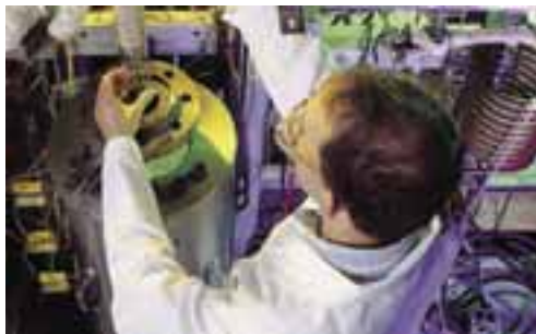
Scientist Brian Turk loads zinc titanate sorbent into a laboratory reactor that removes sulfur from coal gas.
