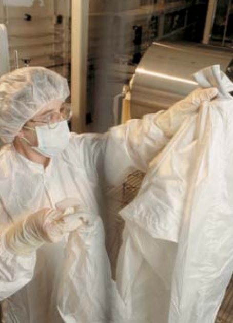
Jenni Elion folds a cleanroom coverall garment for the Helmke drum test, which measures airborne particle shedding.
