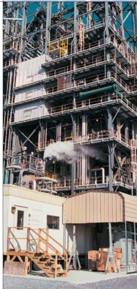
The pilot-scale Direct Sulfur Recovery Process skid and accompanying mobile laboratory, shown in this photo during a field test at the Department of Energy's Power System Development Facility in Wilsonville, Alabama, will be part of the ChevronTexaco project in Southern California.
