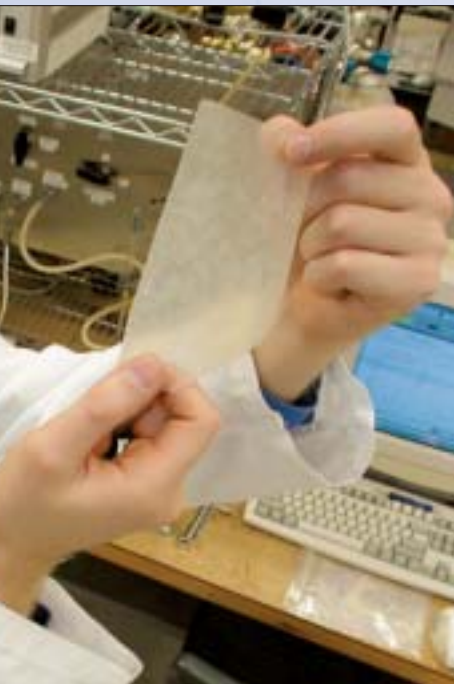
RTI collaborated with NC State University and industry researchers to develop new ultrapermeable, reverse-selective, nanocomposite membranes.
